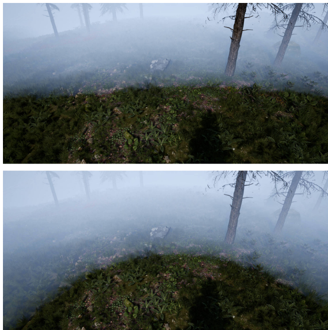
Figure 2: Comparison of fog generation using depth buffer (top) and world/camera position (bottom)
