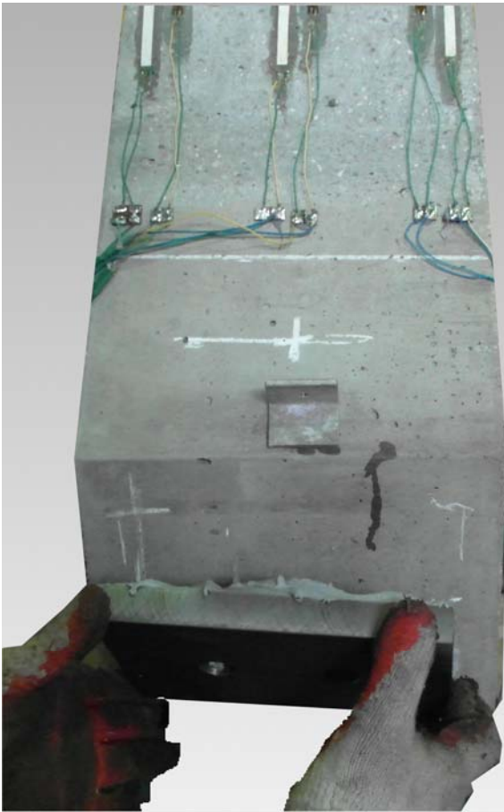
Klejenie blach Gluing the steel plates
