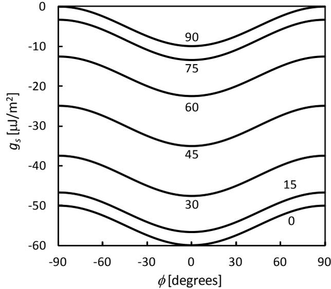
Fig. 1. Anchoring energy density  $g_s$  calculated by use of Eq. (6) as a function of the azimuthal angle  $\phi$  for several values of the angle  $\theta$  (in degrees) indicated at the curves. Planar alignment;  $\mathbf{e} = [1,0,0]$ ,  $W_\theta = 10^{-4} \text{ J/m}^2$ ,  $W_\phi = 2 \cdot 10^{-5} \text{ J/m}^2$
