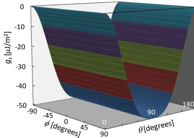
Fig. 5. Anchoring energy density  $g_s$  calculated by use of Eq. (9) as a function of the angles  $\theta$  and  $\phi$ . Homeotropic alignment,  $\theta_s = 90^\circ$ ,  $\phi_s = 0^\circ$ ;  $\mathbf{e} = [0,0,1]$ ,  $W_\theta = 10^{-4} \text{ J/m}^2$ ,  $W_\phi = 2 \cdot 10^{-5} \text{ J/m}^2$
