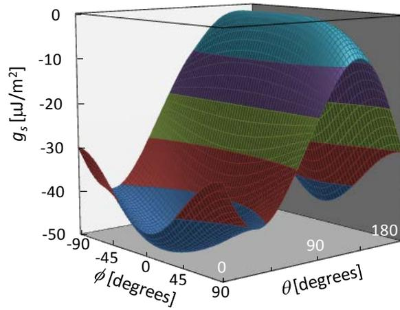
Fig. 4. Anchoring energy density  $g_s$  calculated by use of Eq. (9) as a function of the angles  $\theta$  and  $\phi$ . Oblique alignment,  $\theta_s = 30^\circ$ ,  $\phi_s = 0^\circ$ ;  $W_\theta = 10^{-4} \text{ J/m}^2$ ,  $W_\phi = 2 \cdot 10^{-5} \text{ J/m}^2$
