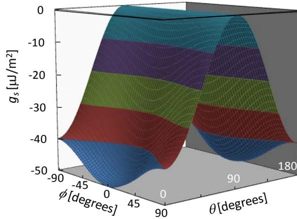
Fig. 3. Anchoring energy density  $g_s$  calculated by use of Eq. (9) as a function of the angles  $\theta$  and  $\phi$ . Planar alignment,  $\theta_s = 0^\circ$ ,  $\phi_s = 0^\circ$ ,  $\mathbf{e} = [1,0,0]$ ,  $W_\theta = 10^{-4} \text{ J/m}^2$ ,  $W_\phi = 2 \cdot 10^{-5} \text{ J/m}^2$
