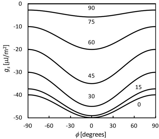
Fig. 2. Anchoring energy density  $g_s$  calculated by use of Eq. (9) as a function of the azimuthal angle  $\phi$  for several values of the angles  $\theta$  (in degrees) indicated at the curves. Planar alignment;  $\mathbf{e} = [1,0,0]$ ,  $W_\theta = 10^{-4} \text{ J/m}^2$ ,  $W_\phi = 2 \cdot 10^{-5} \text{ J/m}^2$
