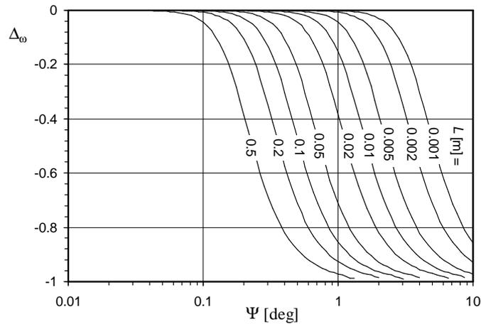
Fig. 2. Relative change  $\Delta_\omega$  in the modulation index caused by the beam divergence  $\Psi$  for various lengths  $L$  of the LiNbO<sub>3</sub> crystal in the configuration  $\sigma = (0,0,1)$  and  $\mathbf{E} = (0,E,0)$ . The absence of any inaccuracies in the crystal cutting and alignment was assumed. The amplitude of the field strength depend on the crystal length  $E_0 = U_0/L$ , where the voltage amplitude on the electrodes is always  $U_0 = 10$  V
