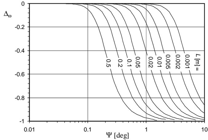
Fig. 1. Relative change  $\Delta_\omega$  in the modulation index caused by the beam divergence  $\Psi$  for various lengths  $L$  of the KDP crystal in the configuration  $\sigma = (0,0,1)$  and  $\mathbf{E} = (0,0,E)$ . The absence of any inaccuracies in the crystal cutting and alignment was assumed. The amplitude of the field strength depend on the crystal length  $E_0 = U_0/L$ , where the voltage amplitude on the electrodes is always  $U_0 = 10$  V
